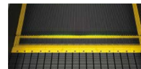
Step demarcation lighting (Shows the step boundaries)
