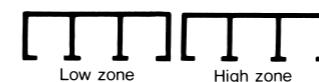
Two banks, in-line arrangement. Inconvenient because of confusion as to the dividing point.
